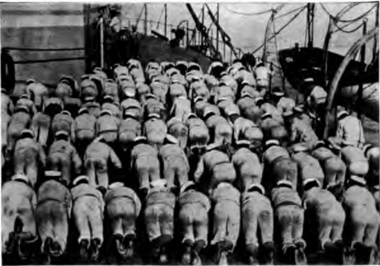
HOLYSTONING A DECK Decks were wetted, then sanded, and bluejackets rubbed them with stones [Page 72]
